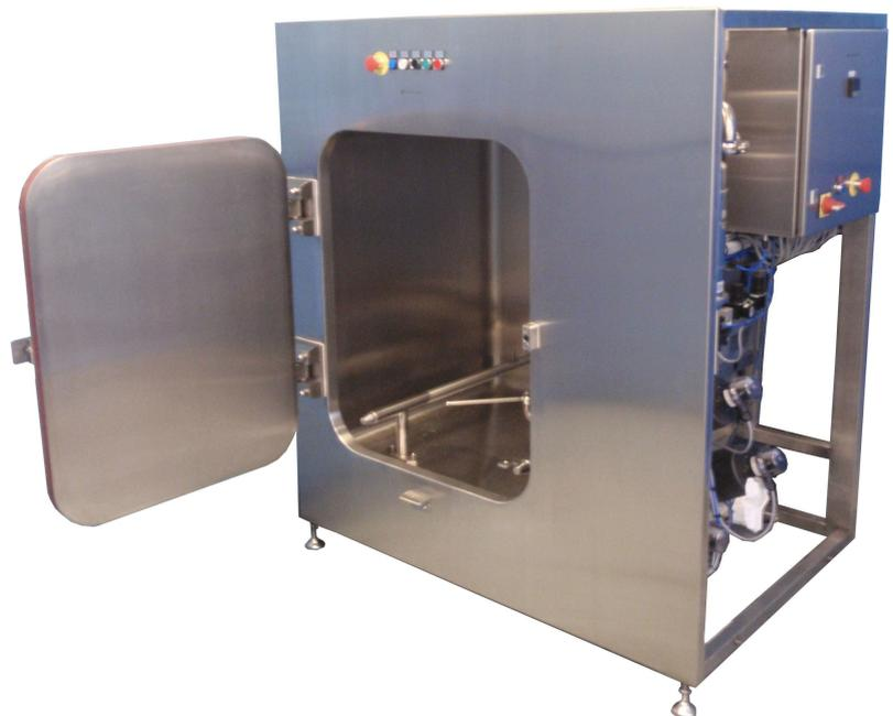
Incorporating crevice free internals, the washers are fitted with an air tight, leak-proof inflatable door seal for total product and washing containment and are available with a single door or two door versions for pass-through requirements. The washers also incorporate standard or bespoke racks
