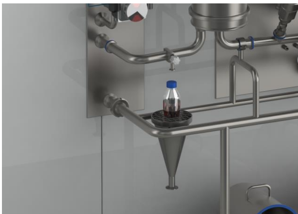
Image 1: Caption 1: Cut of 3D model showing filter skid integrated with Clean Room Panels
