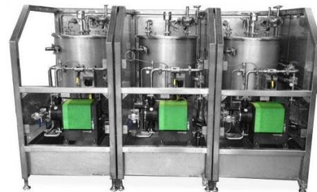
The skids, predominantly used in the pharmaceutical, biotech, healthcare, food and beverage sectors, are designed to meet the high specification and documentation standards required in these industries. The new capacity skids extend the storage capacity to single, twin or triple 1,000 litre storage, with dosing flow-rates of up to 900, 1,800 and 2,700 litres per hour.
