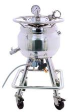
One of the drivers for the transition to single use methodologies is the complexity of the clean in place (CIP) and sterilise in place (SIP) operations of stainless steel multi use equipment, to ensure that there is no cross contamination and all work is developed in a sterile state. There are many advantages in employing re-usable stainless steel equipment and in order to make this usage more practical, the
