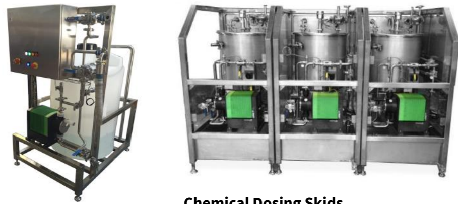
Chemical Dosing Skids
