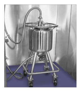
Vessel in Enclosure for SIP
