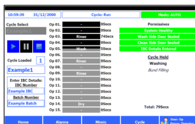
Typical PureCIP™ Operator Interface HMI Recipe Configuration
