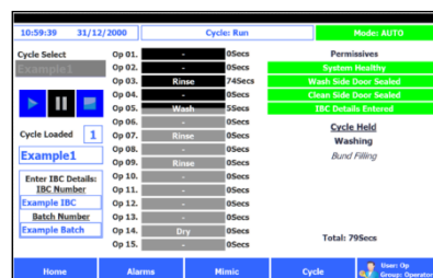
Typical MobileCIPOne™ Operator Interface HMI Recipe Configuration
